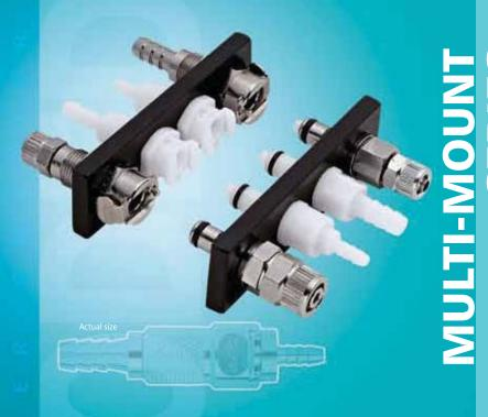
**Multi-Mount couplings** provide one easy-touse coupling for connecting from three to five lines at once. Multi-mount couplings are available in a wide variety of materials including acetal and chrome-plated brass. Multimounts are keyed to prevent mismatched connections and can be configured with or without valves for maximum design flexibility.
