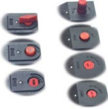
**Overrides** Four types of overrides are available: Standard, Suffix Detail -G, -M and -CML. The standard is a push twist to lock, requires no call out. -G is a guarded momentary contact, -M is an unguarded momentary contact and -CML is a raised grip, push twist to lock.
