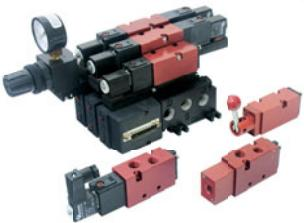
**The C7** is a four-way manifold mounted and body ported, two/three position (5/2 5/3) valve, with  $\frac{1}{4}$ " NPT ports standard and ISO G thread optional. The manifold mounted valves are designed to be mounted on a stacking style manifold and can be manual, pilot or electrically operated with a variety coil options, as well as the Plug-In feature. An optional Pre-Wired sub D connector can support up to 12 valves on a manifold.
