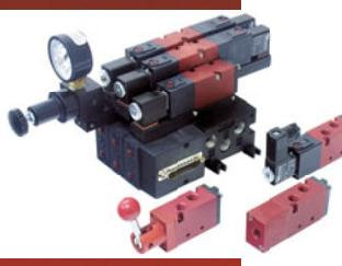
**The C5** is a four-way manifold mounted and body ported, two/three position (5/2 5/3) valve, with  $\frac{1}{8}$ " NPT ports standard and ISO G thread optional. The manifold mounted valves are designed to be mounted on a stacking style manifold and can be manual, pilot or electrically operated with a variety coil options, as well as the Plug-In feature. An optional Pre-Wired sub D connector can support up to 12 valves on a manifold.
