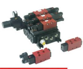
**The C9** is a four-way manifold mounted and body ported, two/three position (5/2 5/3) valve, with  $\frac{1}{2}$ " NPT ports standard and ISO G thread optional. The manifold mounted valves are designed to be mounted on a stacking style manifold and can be electrically operated with a variety coil options, as well as the Plug-In feature. An optional Pre-Wired Amphonal 19 pin connector can support up to 8 valves on a manifold.
